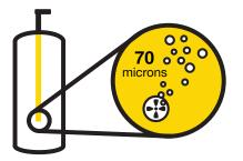
First, the Multi-Rotors located within the **system turn water into droplets of 40-80 micron** size by mixing it with air in a pre-set proportion.
